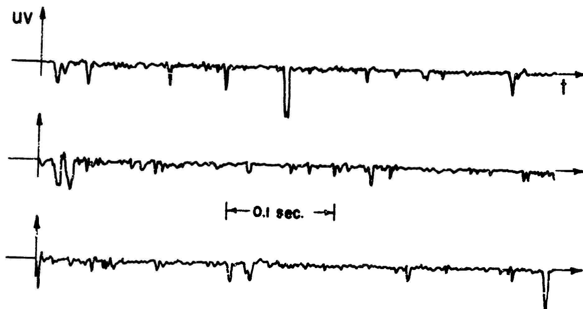
Fig.13 The signal uv as a function of time at y^+ = 30 in low speed boundary layer, U_\infty = 19.7 ft/sec.
