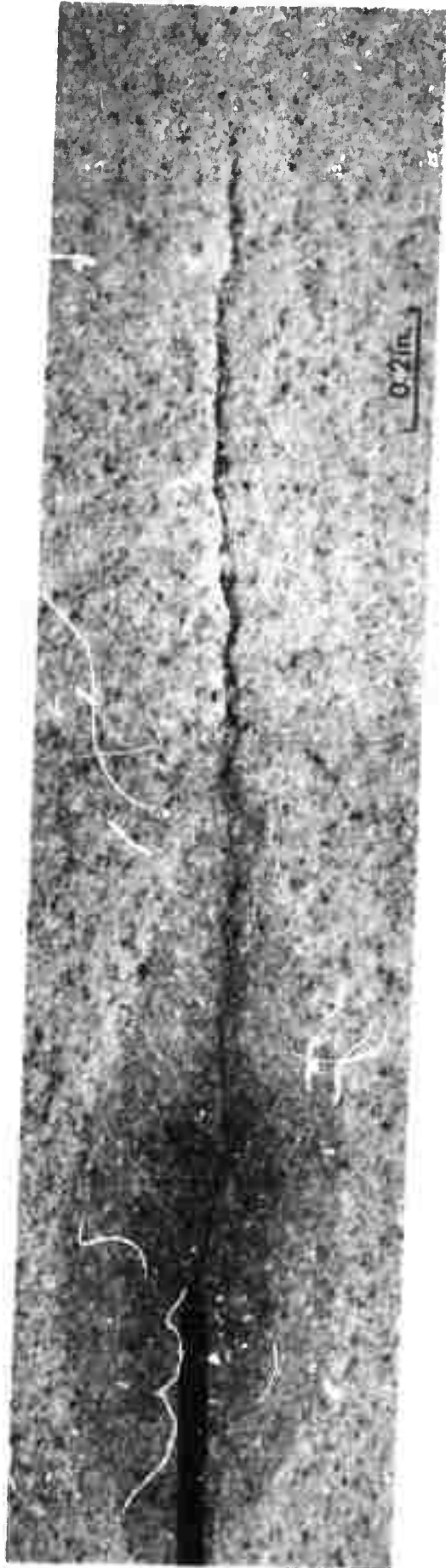
FIGURE 10. CRACK PROFILES AT THE MIDTHICKNESS PLANE OF A BEREA SANDSTONE SPECIMEN. The specimen has been impregnated with an epoxy resin. Note the elliptical zone of penetration of the resin surrounding the slot tip.
