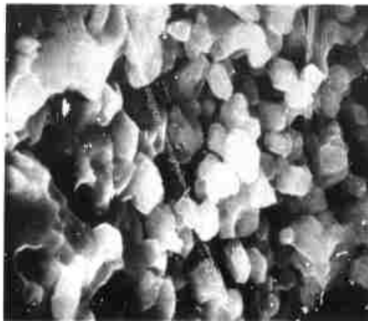
(c) More detail of the fine interöolite aggregate on the fracture surface. (5000X)
