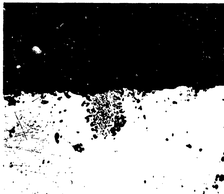
Figure 14. a) Fracture face in billet 642-2 of specimen having oblong flaw, and b) polished face normal to fracture face.
