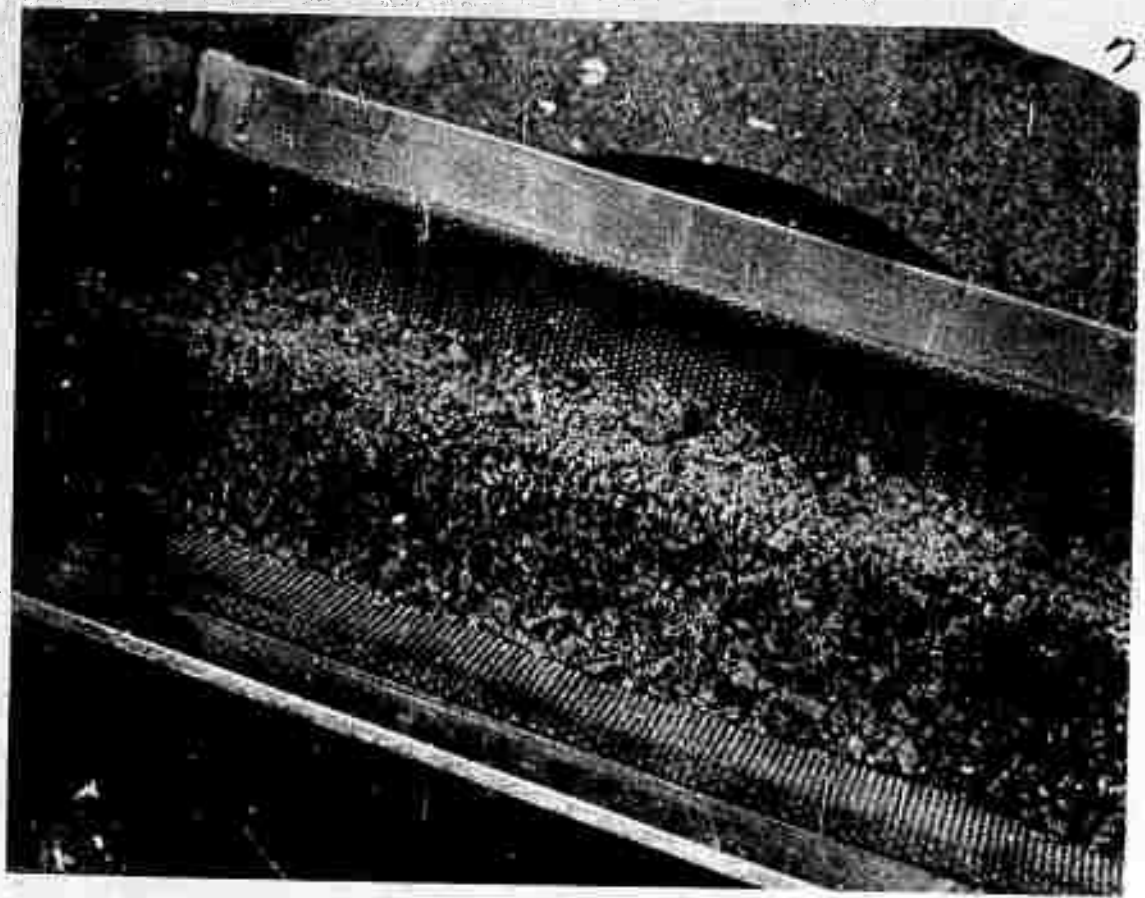
Fig. 6 Bulk material at angle of repose prior to testing
