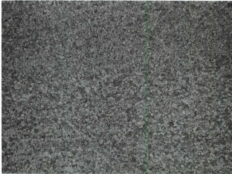
Figure 3 Typical microstructure of Billet #1 (100X).
