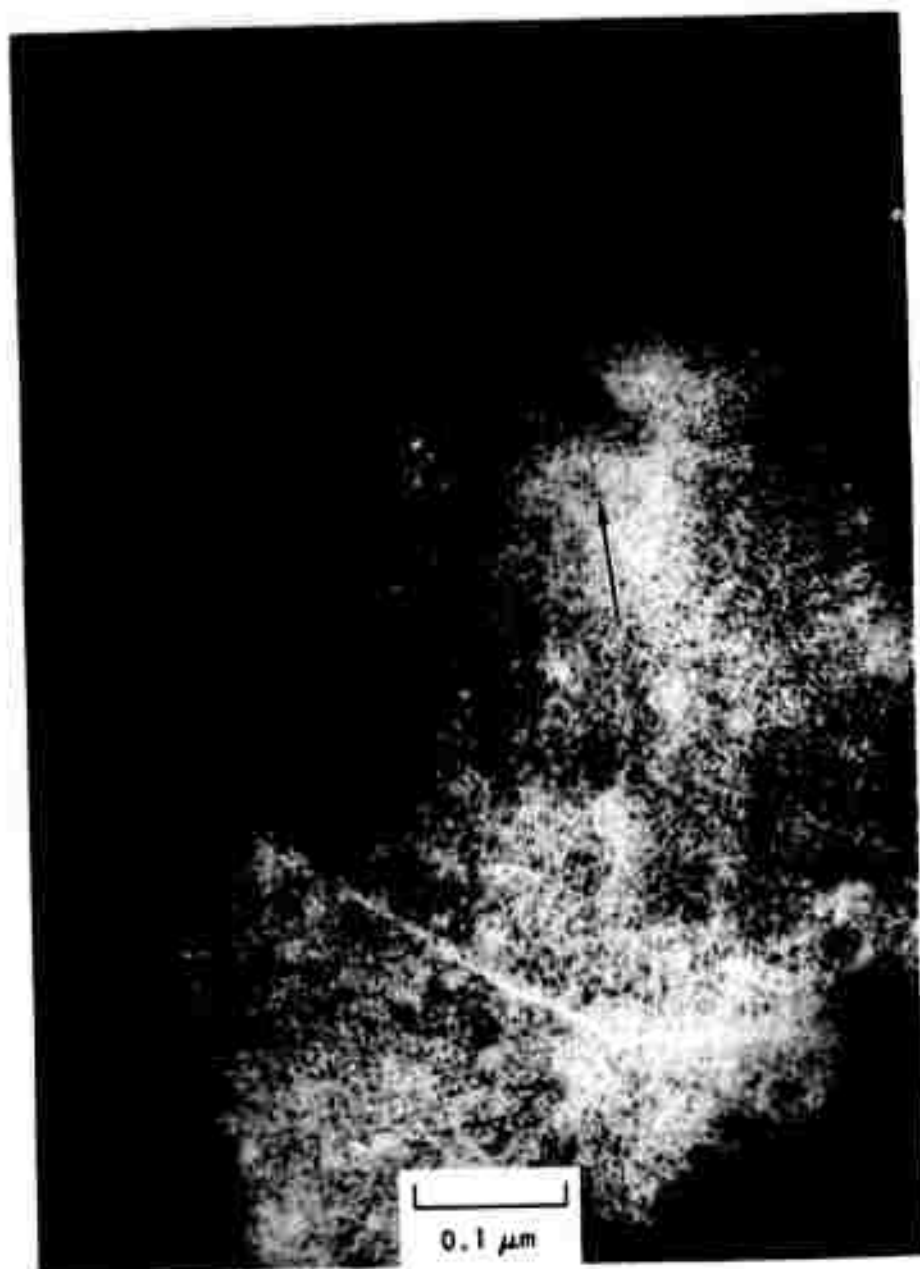
Fig. 14. Transmission electron micrograph of high-density isotropic carbon ( \rho = 1.97 \text{ g/cm}^3 ); sample parallel to the deposition plane. Arrow indicates round particles probably acting as nuclei.
