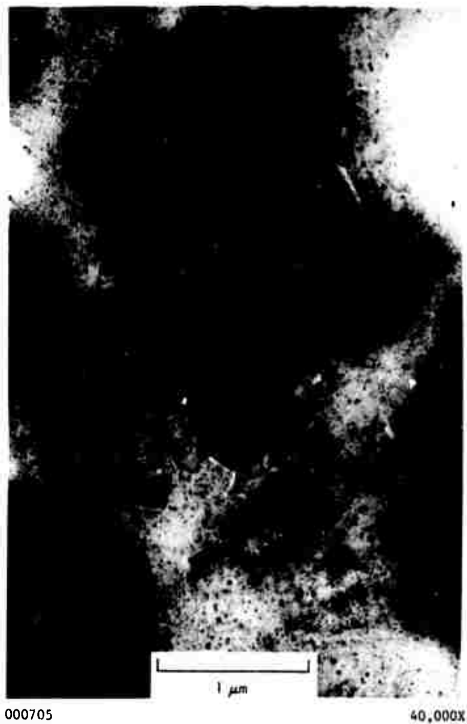
Fig. 16. Transmission electron micrograph of isotropic pyrolytic carbon containing 8 wt-% silicon; sample perpendicular to the deposition plane. Small dark particles are silicon carbide.
