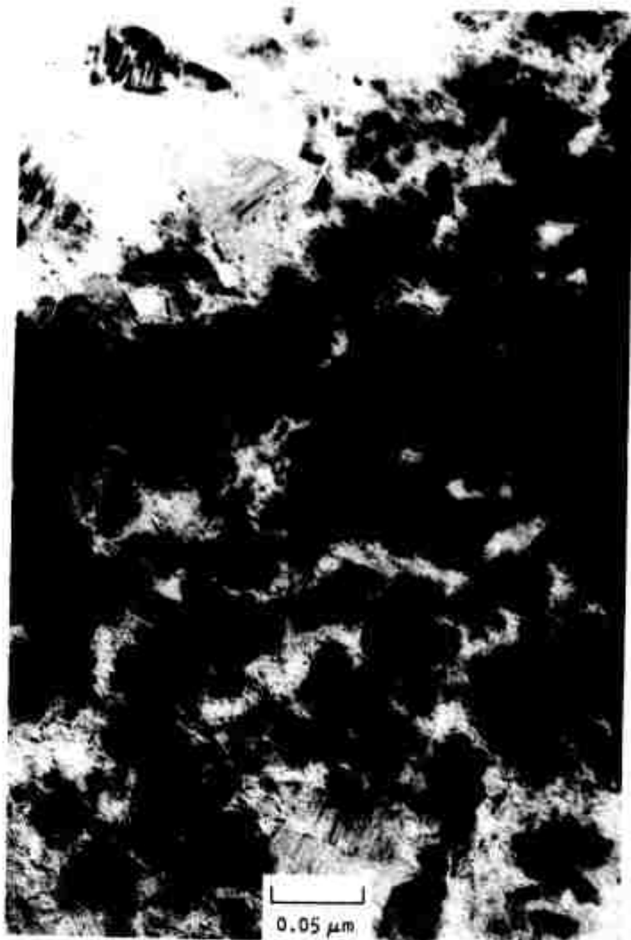
Fig. 18. Transmission electron micrograph of isotropic pyrolytic carbon containing 34 wt-% silicon; sample perpendicular to the deposition plane. Region contains many silicon carbide platelets.
