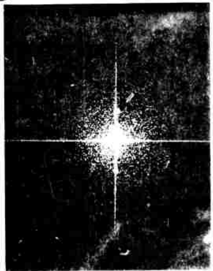
Fig.4 a) Acetate peel of Barre Granite, no load. b) Transform of a); no preferred orientation. c) Acetate peel of same slice as in a) under cantilever load (tension: left-right; load back and forth). d) Transform of c); elongated horizontally, especially in low-frequency range. Scales: a) and c) - Magnification 3.75X ; b) and d) 10 mm corresponds to 1 line/6.75 mm in a) and c).
