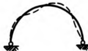
Figure 5.10. Deflection modes of a hinged arch.
