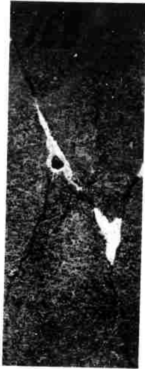
Figure 30 - Photograph of a fatigued Indiana limestone specimen.
