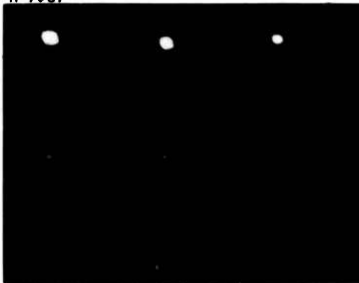
Fig. 1-10. Multiple Lens Camera Photographs of Beam Profile Inside Sapphire Sample for Dif- ferent Incident Energies and Arbitrary Relative Exposures.
