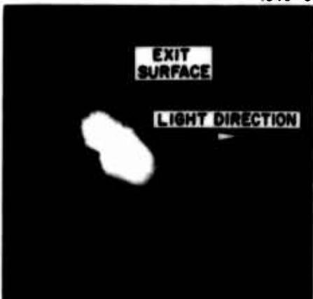
Fig. 10. Time Integrated Photograph of Exit Plasma at Sapphire Surface Tilted 45^\circ With Respect to Light Propagation Direction.
