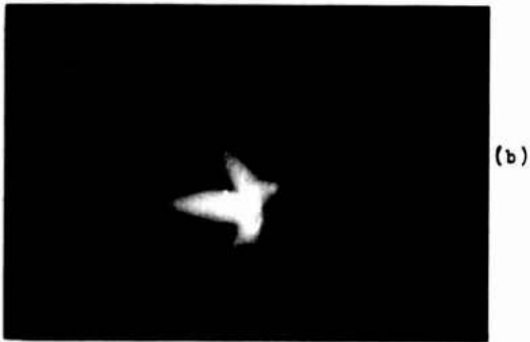
Fig. 9. Time Integrated Photographs of Entrance Plasma at Sapphire Surface Tilted With Respect to Incident Beam Direction. Angle Between Light Direction and Surface Normal (a) 45^\circ , (b) 60^\circ .
