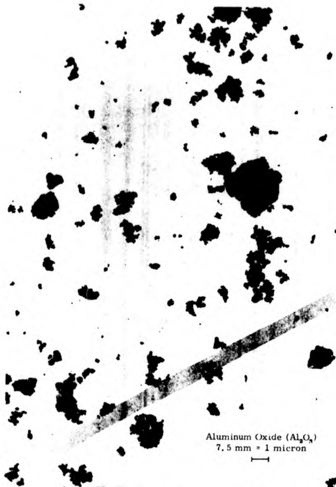
FIG. 1. ELECTRON PHOTOMICROGRAPH OF ALUMINUM OXIDE (Al 2 O 3 ) Vendor Specification, 0.3 \mu
