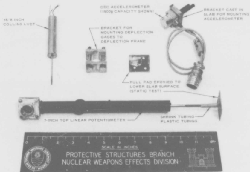
Figure 3.38 Acceleration and deflection transducers.
