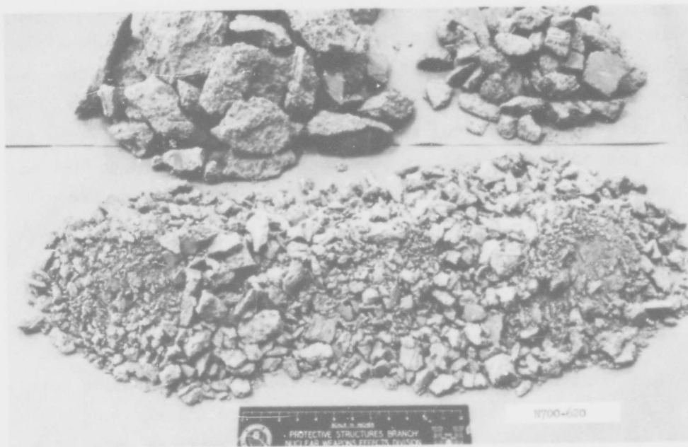
Figure 6.11 Debris from the southwest column area, Dynamic Test II.
