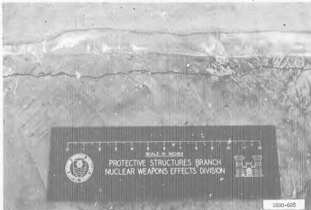
Figure 4.16 Crack over inner wall face, north side of specimen after Dynamic Test I.
