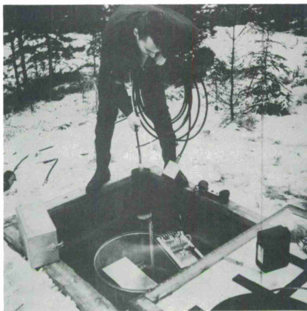
Figure 4.9 Technician lowering an SP seismometer down into the bore hole.
