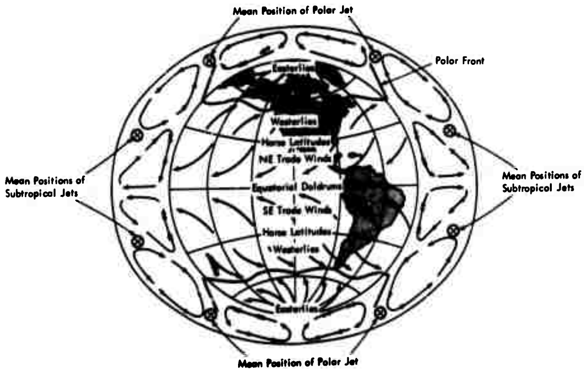
FIGURE 5. Schematic Representation of the General Circulation within the Troposphere for Current Climate (Miller & Thompson, 1970)
