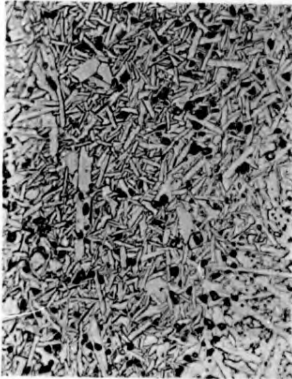
Fig. 18 - SiC R-48, X1000, thermal etch. Moderate case of exaggerated grain growth.
