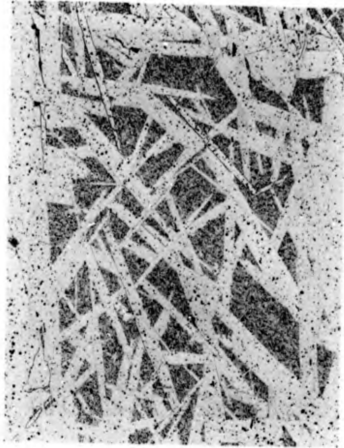
Fig. 12 - SiC R-74, 100X, thermal etc. Impinging and interpenetrating tabular crystals. Trapped pores.
