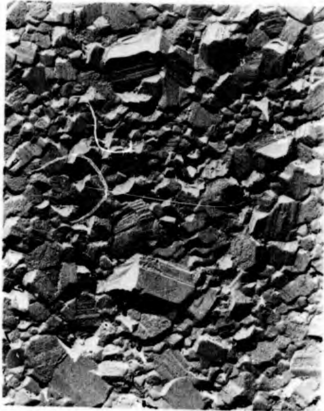
Fig. 15 - SiC R-42, 30,000X, thermal etch, double-stage replica. Equiaxed uniform grains typical for oxygen-rich powders. Note traces of twin boundaries.
