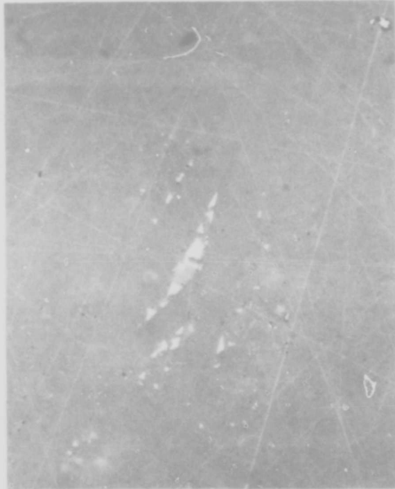
Fig. 11 - SiC R-59 as polished, 1500X. Silicon phase in the vicinity of large tabular grains of SiC.
