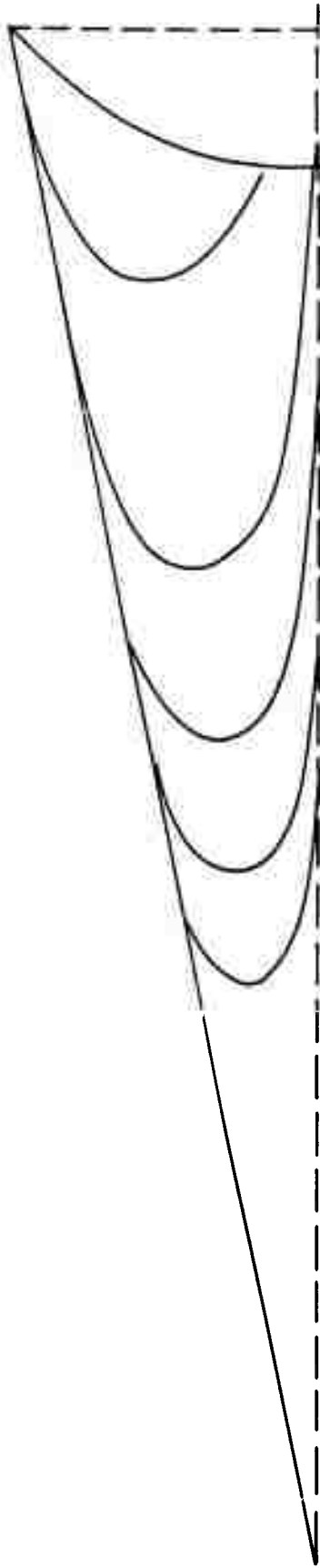
FIG.10: STREAMLINE IN HALF-CONE FOR FRAME AT REST IN CONE
