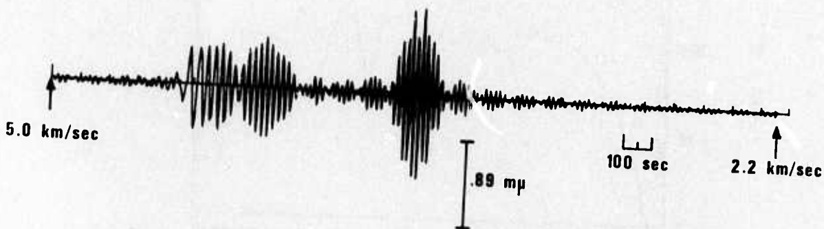
Figure 8d. Seismograms for 1 kT yield and \Delta = 10000 km for different source types, source altitudes, and earth models. Oceanic models, source at 1.83 km. In each case the upper seismogram for a mass-injection source, the middle seismogram for an energy-injection source, and the lower seismogram for a surface overpressure source.
