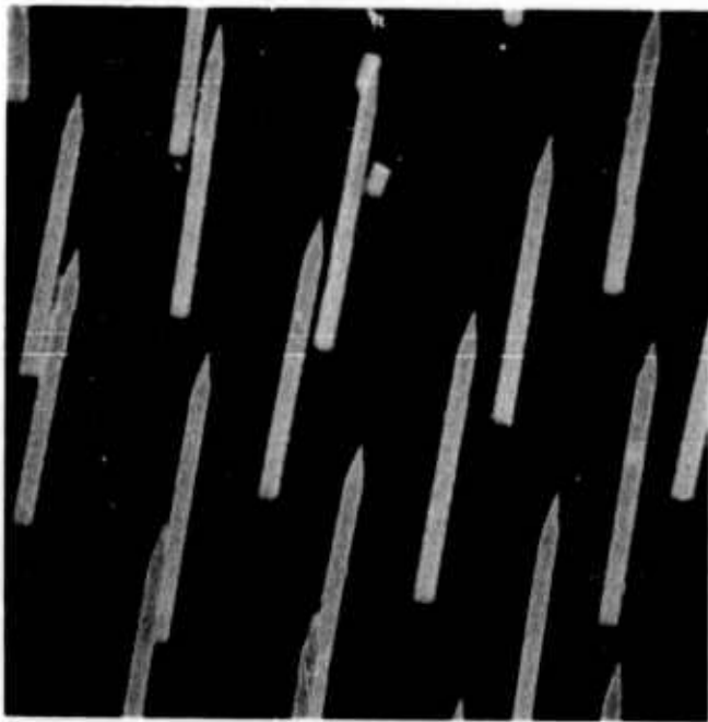
Figure 1. Scanning Electron Micrograph of UO_2 -W Composite Containing Approximately 1.5 w/o W Displaying Widely Spaced Fibers.
