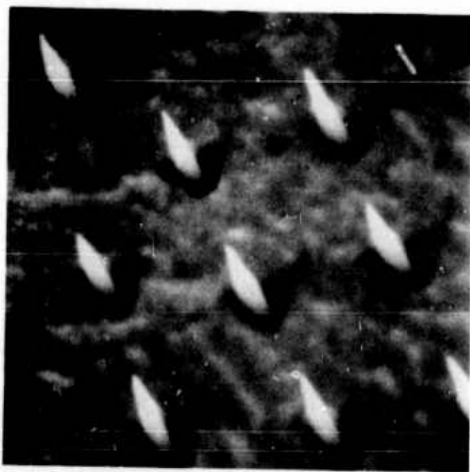
Figure 24. \text{UO}_2 -W Composite Displaying Blunter Points Obtained by Reducing \text{CrO}_3 Solution Content from 20 to 15 ml. Etching Was Performed at 0^\circ\text{C} With HF Content of 10.0 ml. Scanning Electron Micrograph, X13,000.
