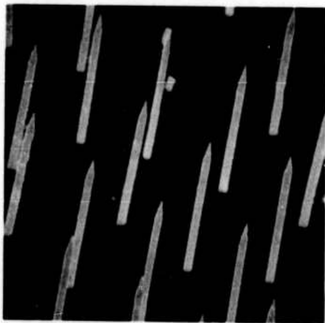
Figure 30. UO 2 -W Composite (Sample No. 25-49) Showing Results Obtained by Lengthening Etch at Room Temperature Rotating Sample at 20 rpm. Scanning Electron Micrograph, X6,500.
