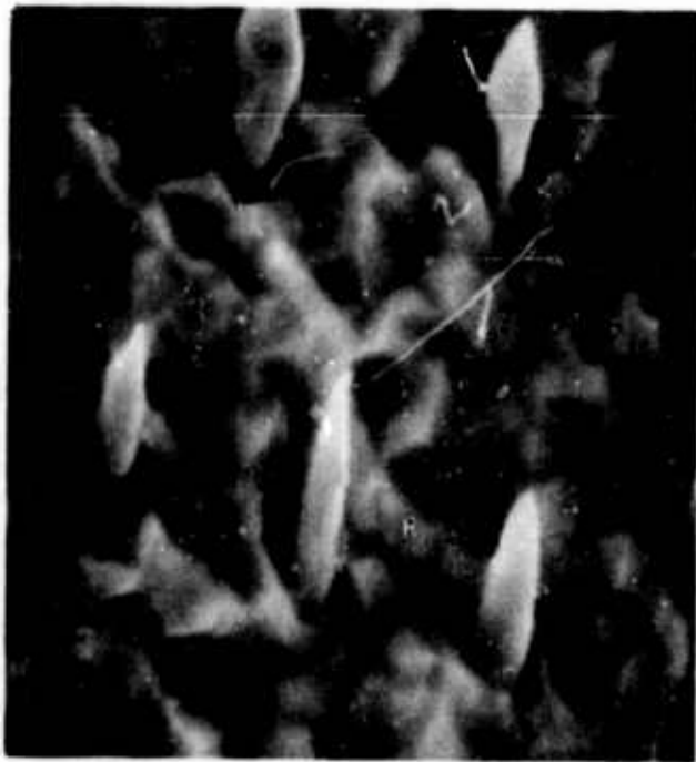
Figure 17. \text{UO}_2 -W Composite Etched at 48^\circ\text{C} in Etchant Containing 5.8 ml HF. Scanning Electron Micrograph, X12,000.
