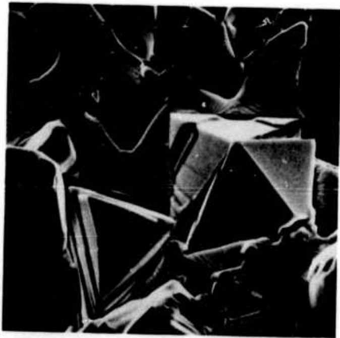
Figure 37. Surface of Platinum Braze Showing Small Crystals and Absence of Fibers. Scanning Electron Micrograph, X2,400.
