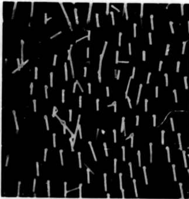
Figure 39. Scanning Electron Micrographs of Two Areas of the Cu Braze Surface Showing W Pins Pulled From the \text{UO}_2 -W Composite. X2,100.
