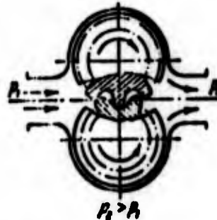
Fig. 1.6. Diagram of a gear pump.
