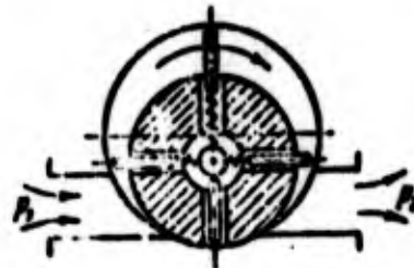
Fig. 1.7. Diagram of a rotary pump.
