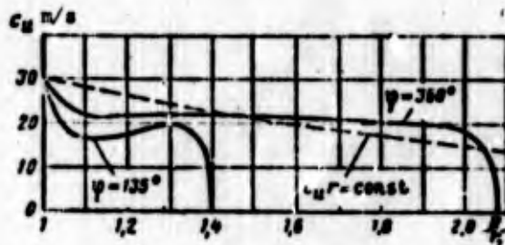
Fig. 3.25. Theoretical (dashed line) and experimental curves of the change in the circular velocity component of the flow c_u along the radius of the spiral collector.
