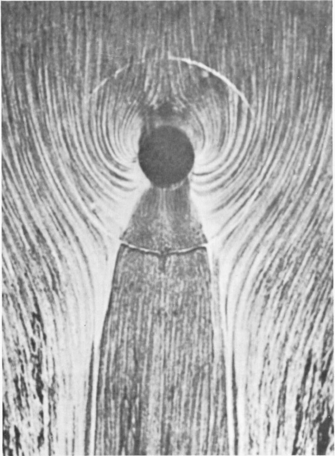
a. Oil-Trace Photograph (Ref. 2) Fig. 3 Flat-Plate Studies, V_j/V_\infty = 8.0
