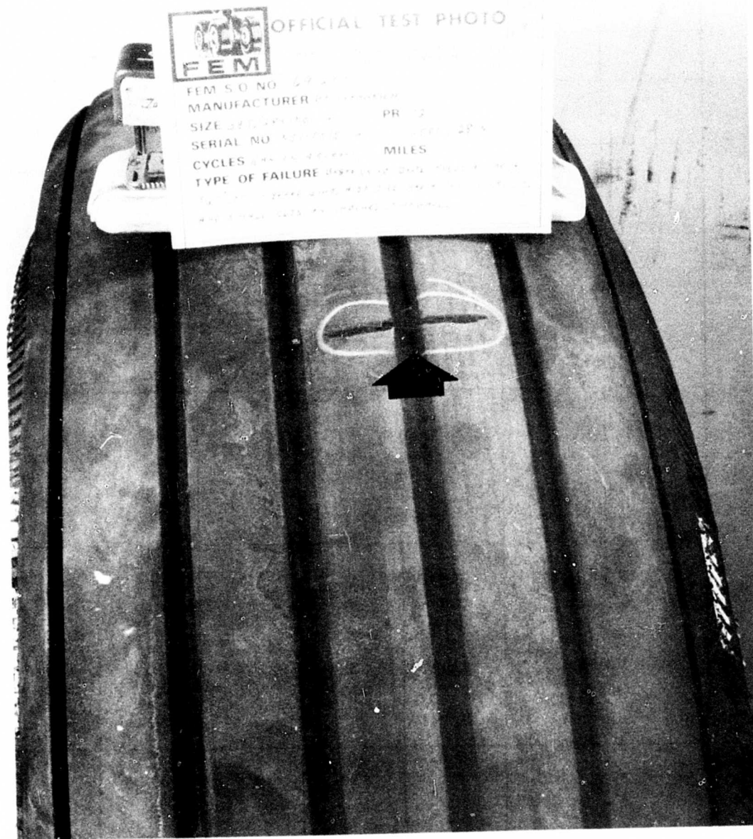
Figure 24. Tread Cut On Tire No N51-0035-16.
