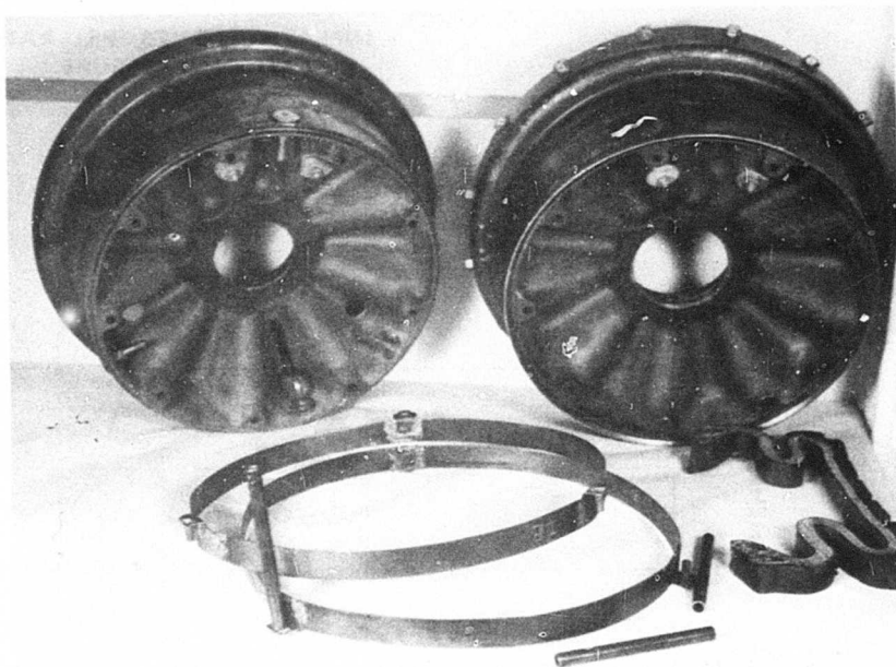
Figure 9a. Wheel and Bead Spacer Components.
