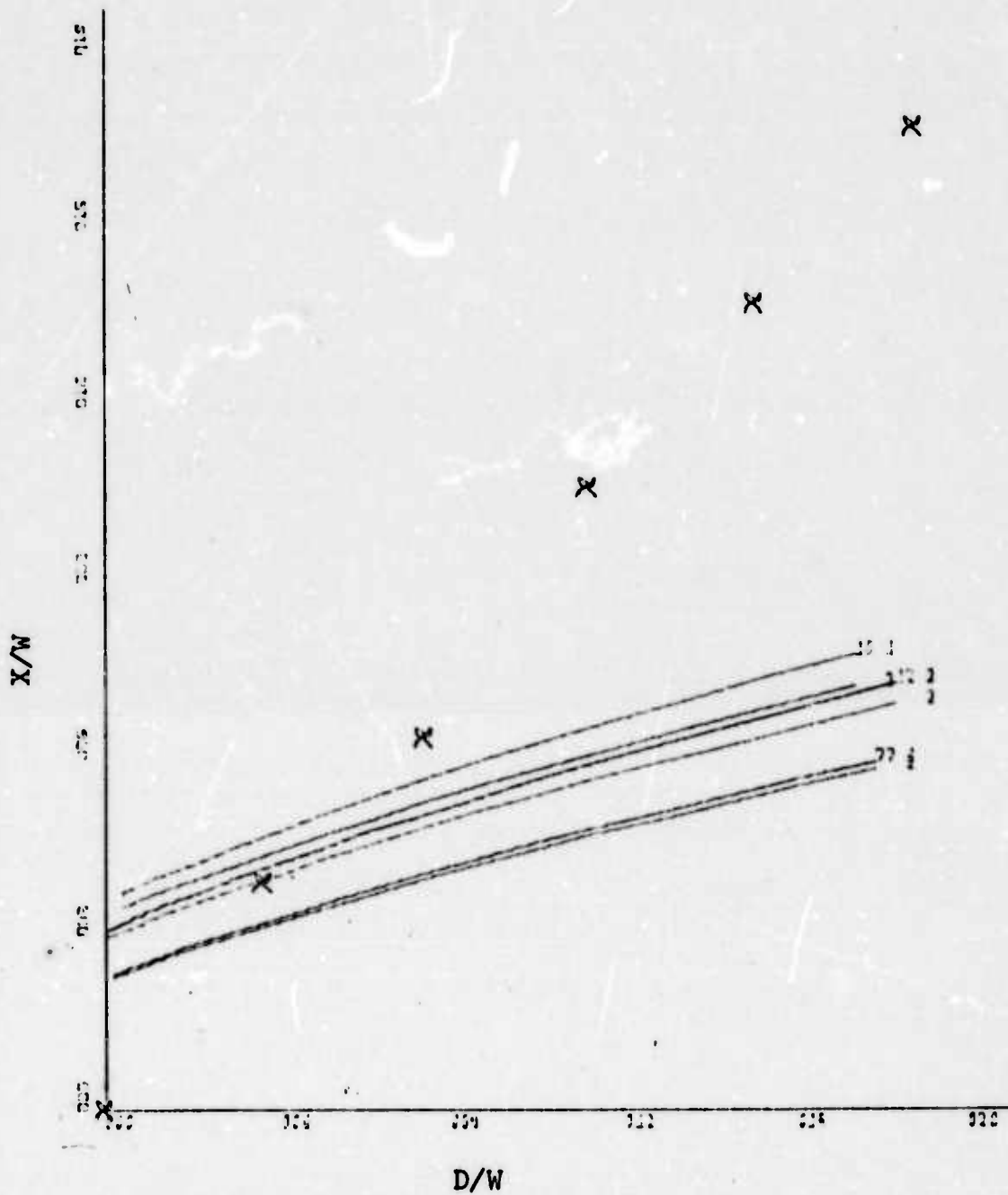
Figure 44. Attachment Distance vs. Offset Distance for a Concave Wall at 20 Degrees Incidence Using Methods One(1) and Two(2) and Comparing With Experimental Data, Jet Width of 1.31 inches, Re = 1.475 \times 10^5 , \sigma = 7.7, 12, 15 .
