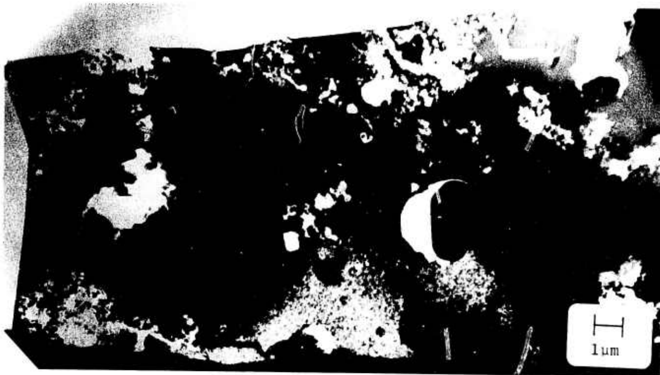
Figure 103. Reaction of Si with \text{Al}_2\text{O}_3 during In Situ Growth
