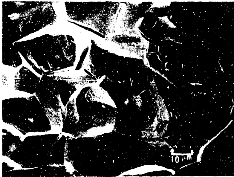
Figure 34. Intergranular fracture surface of unalloyed tungsten.
