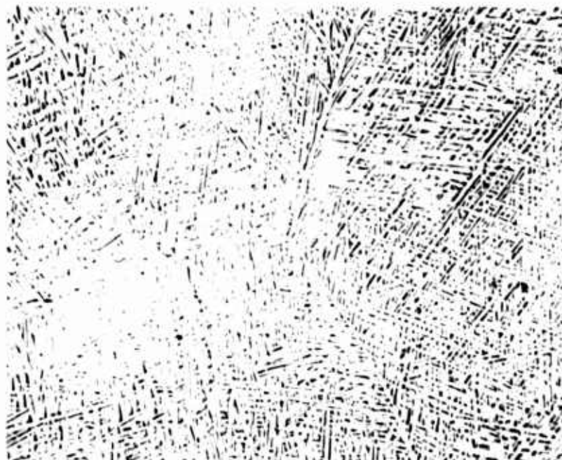
FIGURE 42. SYNTHETIC HEAT-AFFECTED ZONE, 25F/SEC, 1400F - 4 HRS PLUS 500F - 1000 HRS
