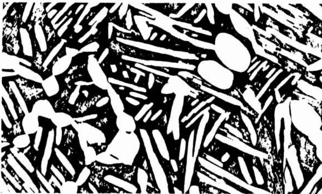
Fig. 20 - Ti-6Al-4V Condition 12, 1-in. plate, 1850°F-½ h-AC, 1750°F-4 h-WQ, 1000°F-2 h-AC. K_{Ic} = 59 \text{ ksi-in}^{\frac{3}{2}} , F_{ty} = 160 \text{ ksi} .
