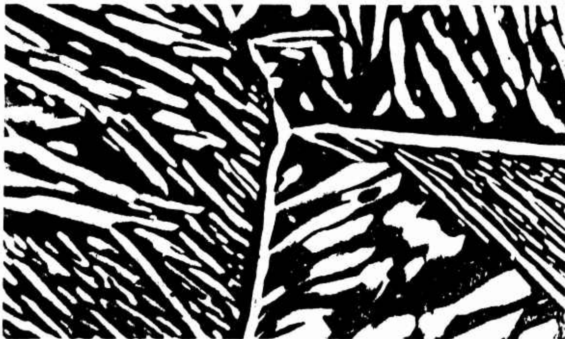
Fig. 22 - Ti-6Al-4V Condition 1a, 1-in. plate, 1875 o F-1 h-AC, 1750 o F-2 h-WQ, 1000 o F-2 h-AC. K_{Ic} = 71 \text{ ksi-in}^{3/2} , F_{ty} = 156 \text{ ksi} .
