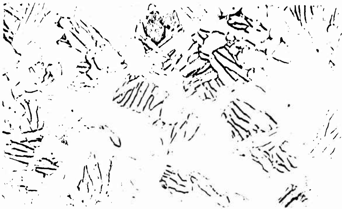
Fig. 35 - Ti-6Al-4V Condition 27, 4- X 4-in. forged billet, \alpha -segregated, equiaxed, 1775 o F- \frac{1}{2} h-AC, 1450 o F-1 h-AC. K_{Ic} = 72 \text{ ksi-in}^{\frac{1}{2}} , F_{ty} = 130 \text{ ksi} .
