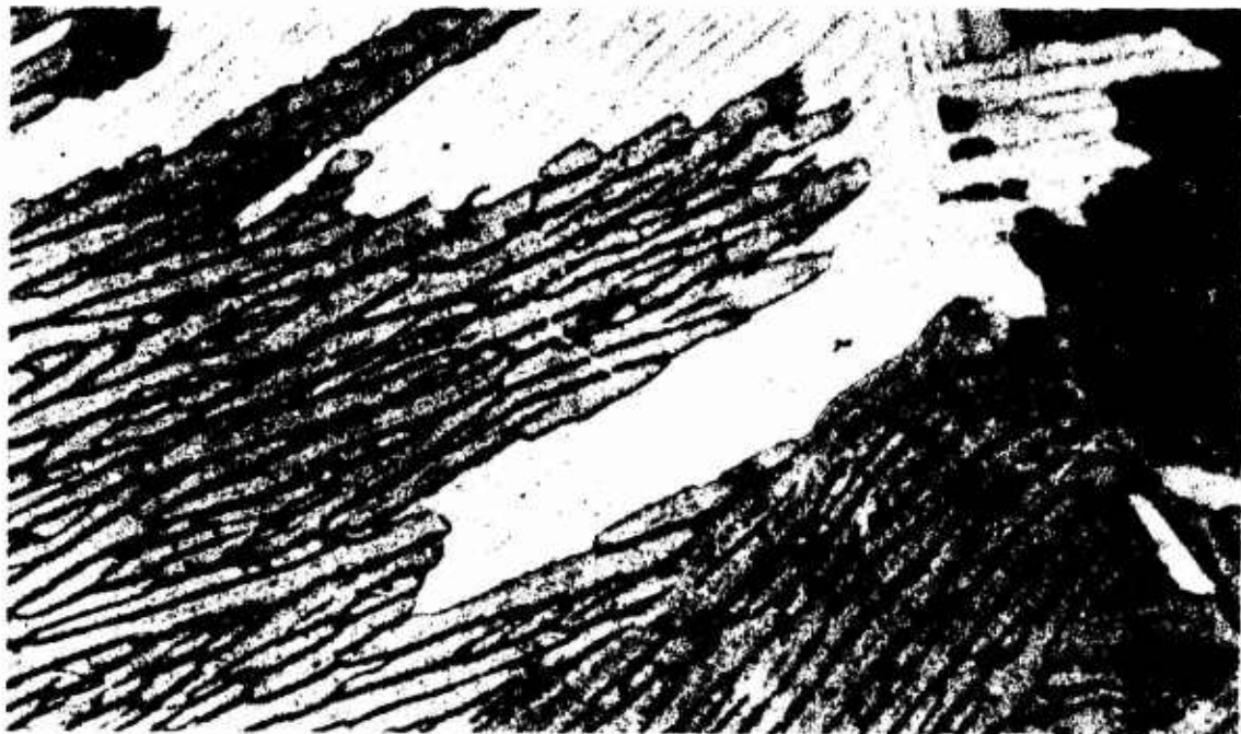
Fig. 21 - Ti-6Al-4V Condition 1s, 1-in. plate, 1875 o F-1 h-AC, 1750 o F-2 h-AC, 1-90 o F-1 h-AC. K_{Ic} = 37 \text{ ksi-in}^{3/2} , F_{ty} = 125 \text{ ksi} .
