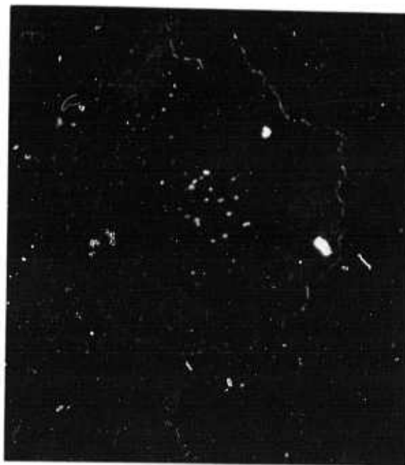
Figure 17. Laser-induced damage far above the spark threshold on a \text{TiO}_2/\text{SiO}_2 multilayer reflector (Sample S101). Random penetrations to deeper layers is apparent. (magnification: 120x)
