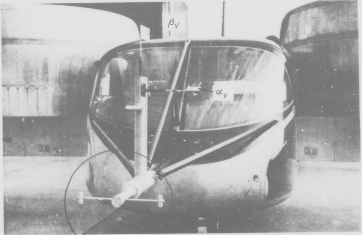
Figure I-15 VERTICAL VELOCITY LORAS INSTALLATION ON NOSE BOOM WITH \alpha AND \beta VARIES
