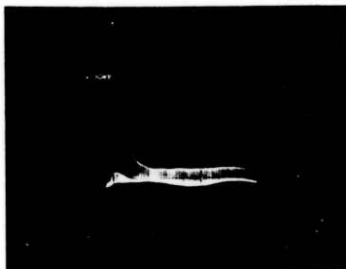
Fig. 9 \text{TEM}_{00} Mode Laser Output (200 ns/cm)
