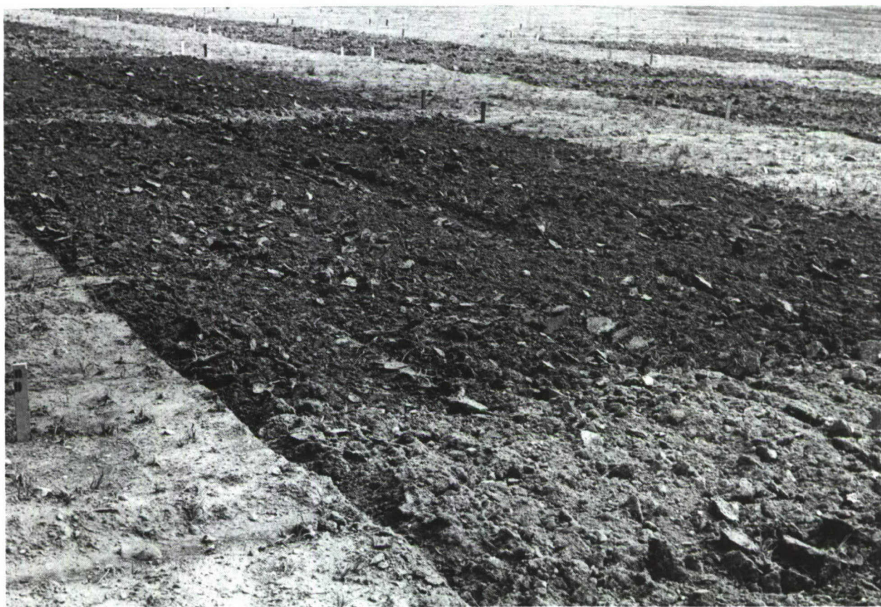
FIGURE 26. Field Test 3 - Soil disced prior to test (same day) - foreground, no mulch; background (dark area), mulched immediately before photographed.
