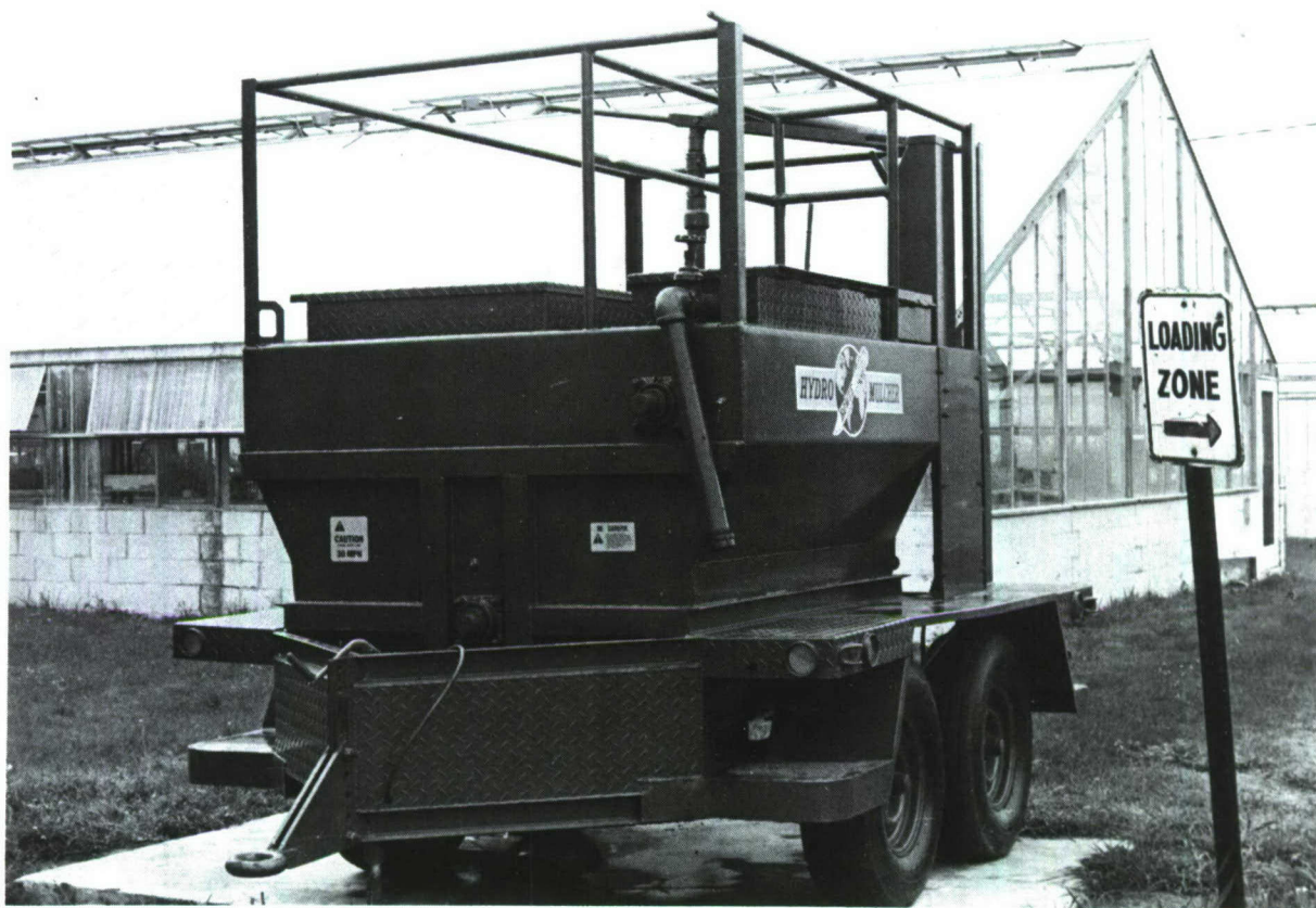
FIGURE 18. Bowie Hydromulcher - 500-gallon Victor model (front).
