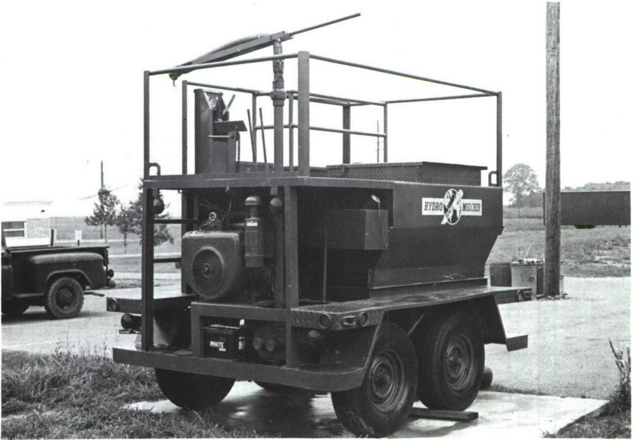
FIGURE 19. Bowie Hydromulcher - 500-gallon Victor model (back).
