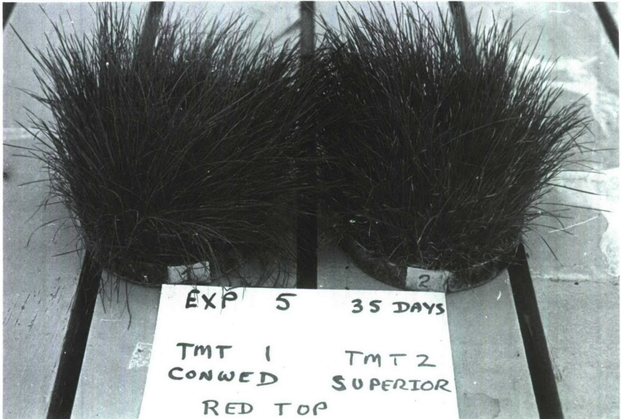
FIGURE 3. Test 5 - Redtop ( Agrostis alba ) after 35 days. The test media was vermiculite with top mulch of Conwed Hydromulch or Superior Hydromulch.
