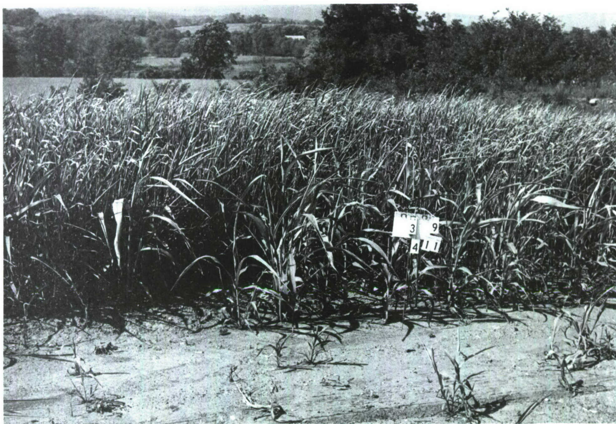
FIGURE 36. Field Test 4 - Plot 3, 53 days after application (before irrigation). 3000 lbs of mulch and Curasol AE. Sorghum-sudan, rape and Proso millet.
