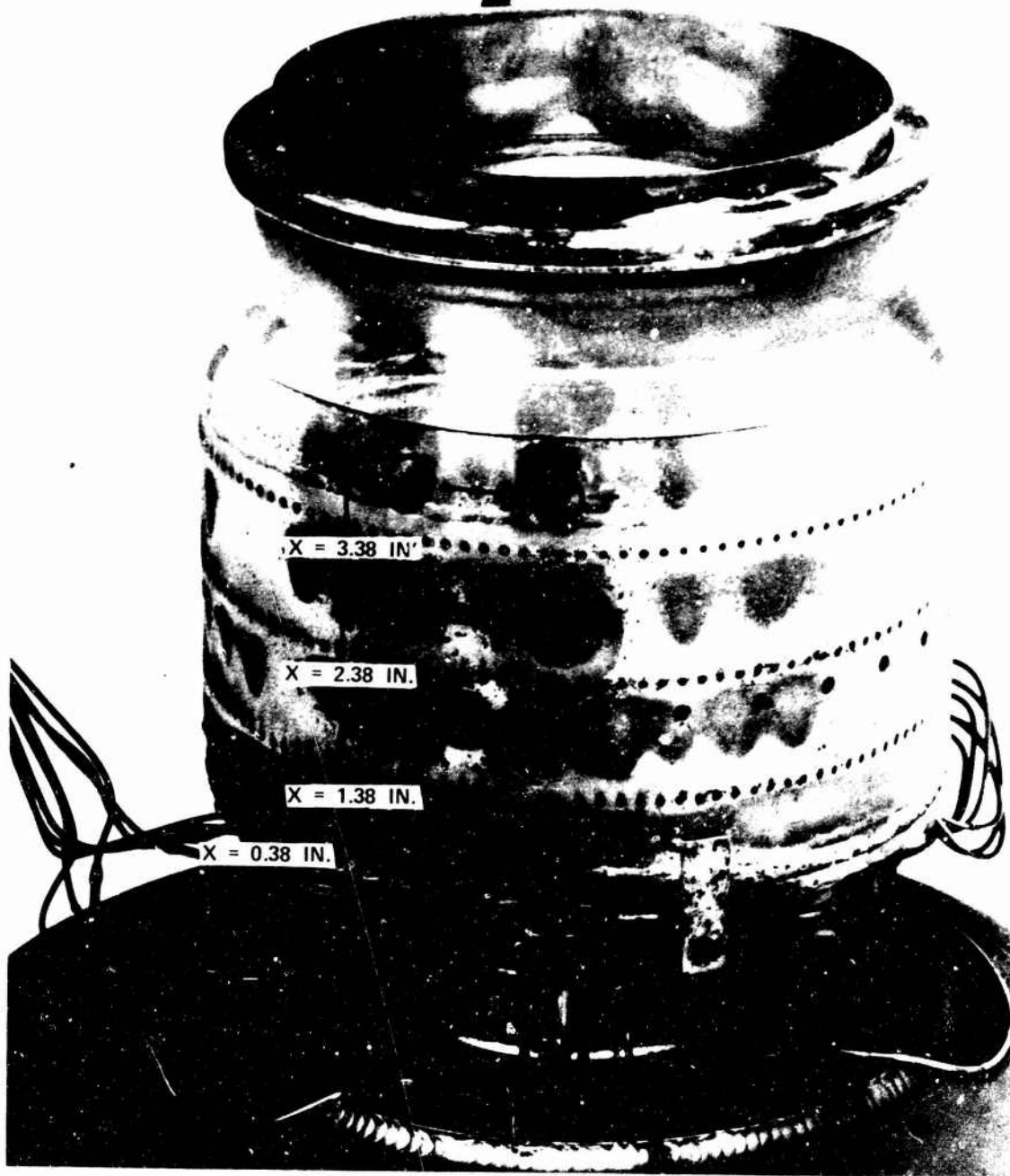
Figure 23. Combustor Cold-Flow Mapping Ports (After Weld Repair).
