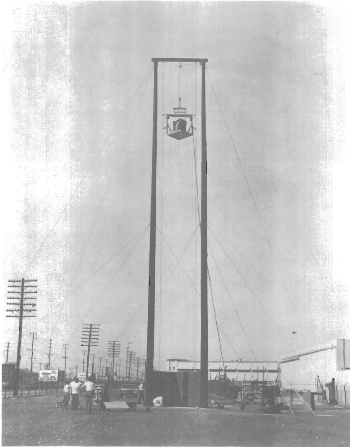
Figure 13. Tower With Test Tank Aloft.
