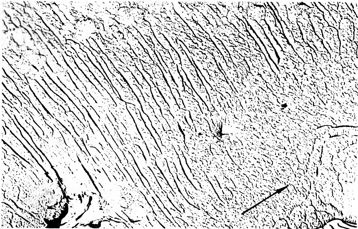
Fig.2 Fatigue fracture in a mild steel after smoothing and electrolytic attack. Network of dislocation walls perpendicular to the propagation direction indicated by the arrow.
