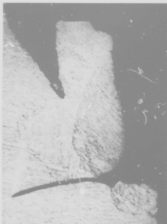
Fig.20 Maraging steel, cleavage and intergranular fracture. X1000
