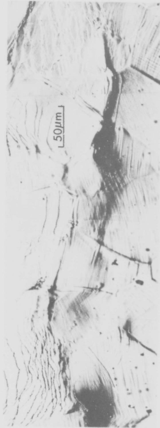
Fig.4.8 Optical micrographs of replicas of the surface of a plastically bent strip showing the progressive development with plastic strain of a super band in a 7000-series alloy in the peak aged condition. The tensile direction is vertical. (a) plastic strain 0.08, (b) plastic strain 0.17
