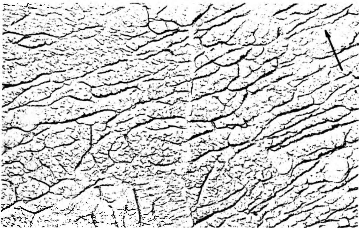
Fig.3 Field close to Figure 2, observed on both sides of a grain boundary a few dislocation cells appear clearly on this picture
