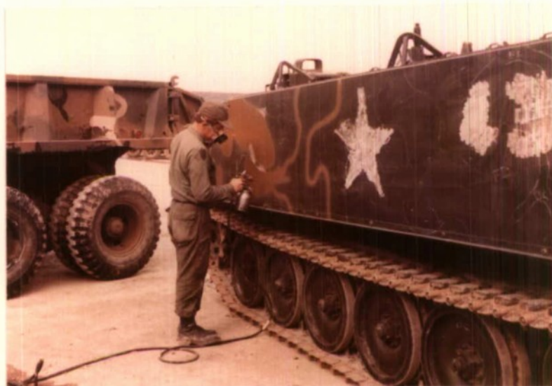
Fig. 7. Soldier outlining the pattern in the color to be painted. This method provides a boundary and controls the painting within its limits.
