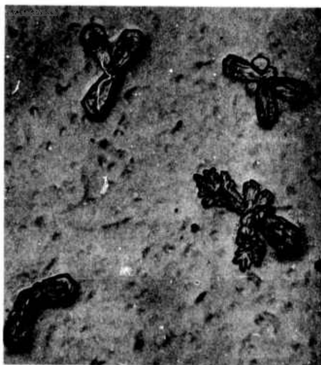
Figure 54 ICE CRYSTAL REPLICAS AND PARTICLES LOCATED WITHIN THEM
