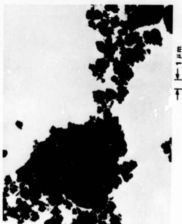
Figure 3 CLAY SPRINKLED ON A PREPARED TEM GRID
