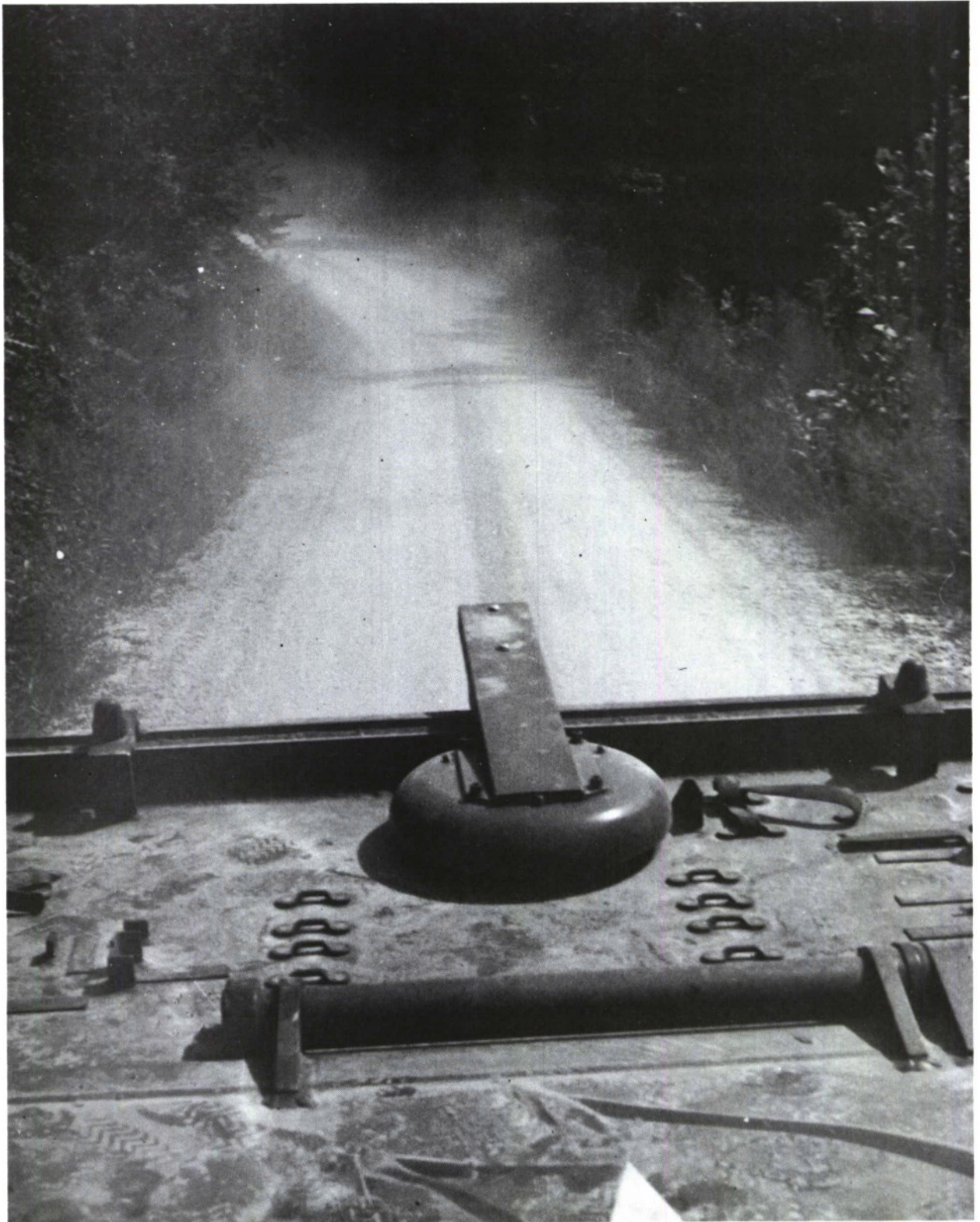
FIGURE 5-2. COMPASS MOUNTED ON APC
