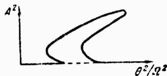
Figure 4.6. The "amplitude-frequency" curve for parametric vibrations of a circular cylindrical shell.
