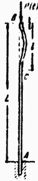
Figure 6.4. Char- acter of buck- ling of a com- pres- sed bar under im- pact.
