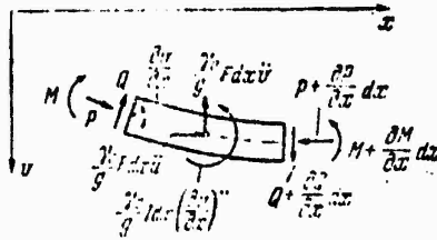
Figure 8.2. Concerning the derivation of equations for longitudinal-transverse motion of the bar.
