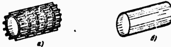
Figure 7.22. Circular cylindrical shell: a) reinforced with stringers and ring frame supports; b) smooth.
