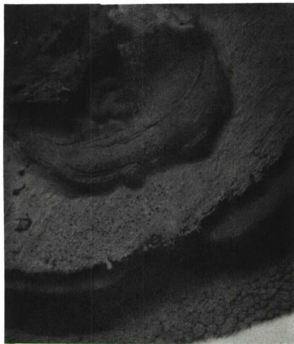
FIGURE 35 SCANNING ELECTRON MICROSCOPE PHOTOGRAPHS OF A PHS CONSTRUCTION GUNN DIODE FOLLOWING FAILURE. THE TOP STRAPS HAVE BEEN REMOVED, REVEALING THE FAILURE REGION. CRACKING AT THE EDGES POSSIBLY DUE TO STRESS FROM THE PLATED GOLD HEAT SINK IS SHOWN.
