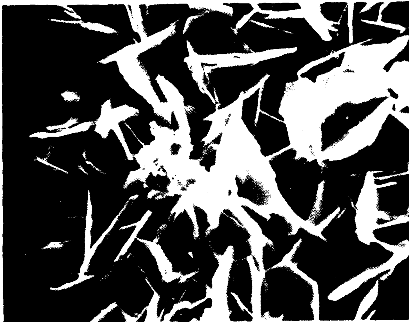
FIGURE 13. ZINC, 28 DAY QUIET SEA WATER EXPOSURE, 600X
