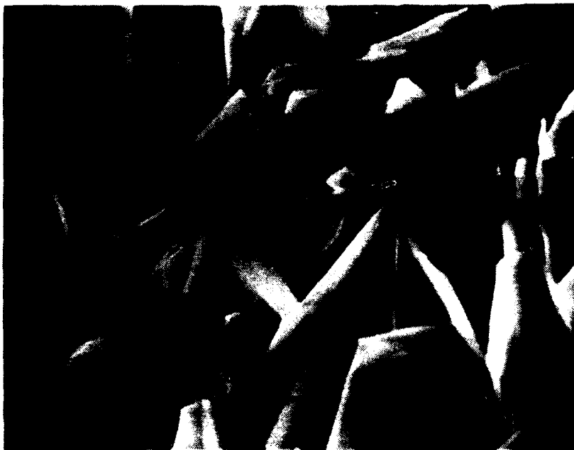
FIGURE 23. ZINC, 7 DAY QUIET SEA WATER EXPOSURE 89 PSI, 2300X
