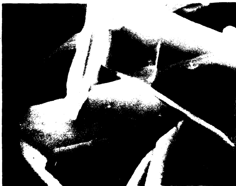
FIGURE 16. ZINC, 21 DAY QUIET SEA WATER EXPOSURE, 2400X
