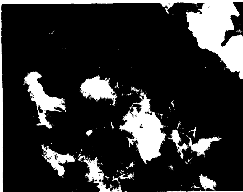
FIGURE 28. ZINC, ANODIC POLARIZATION, 5 MIN. AT 1000MA, -0.5V, 2400X
