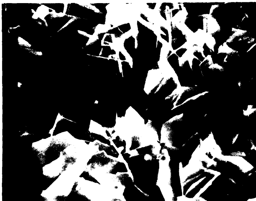
FIGURE 15. ZINC, 14 DAY QUIET SEA WATER EXPOSURE, 620X
