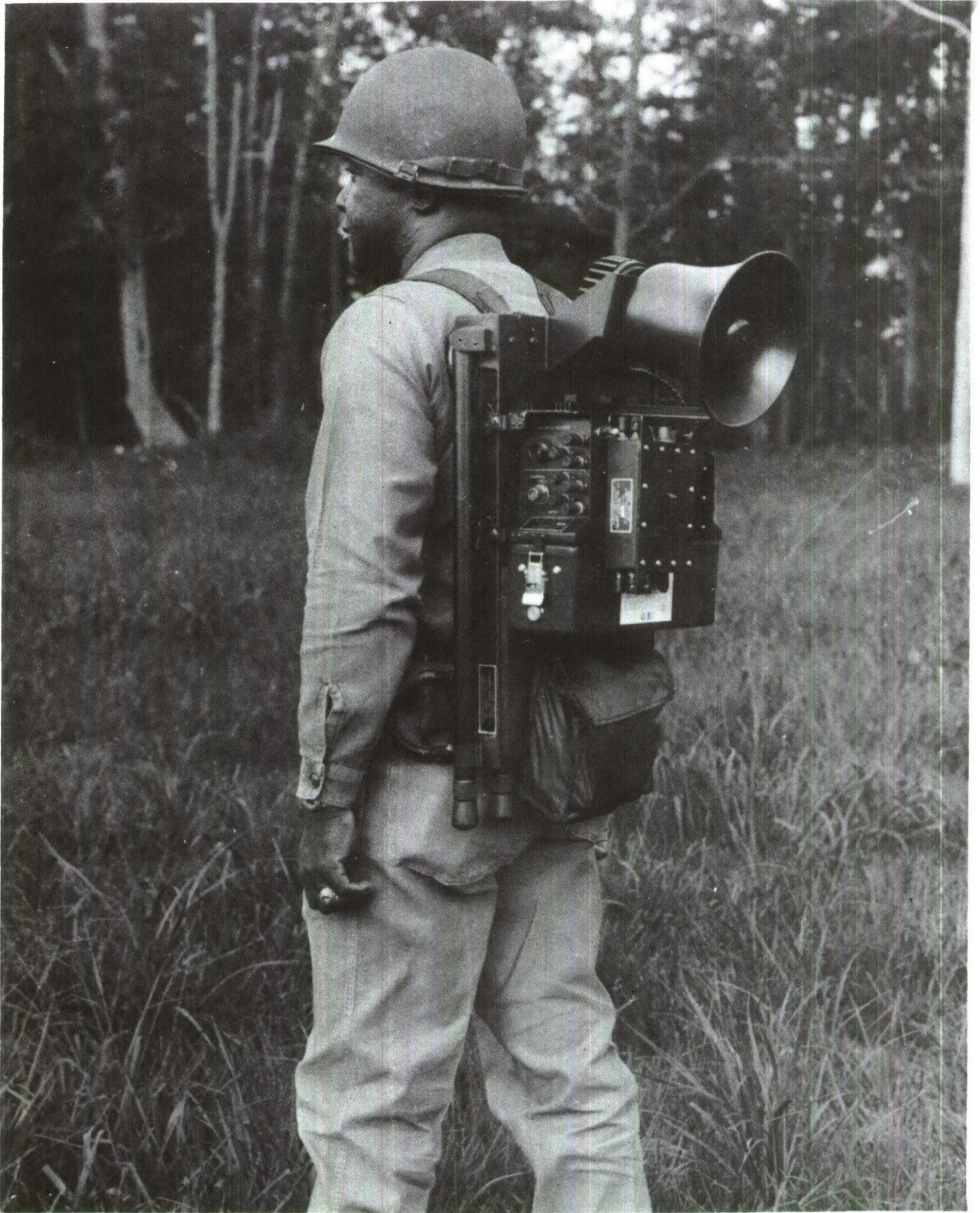
Figure 3. Public Address Set AN/UIQ-11 Shown Backpacked
