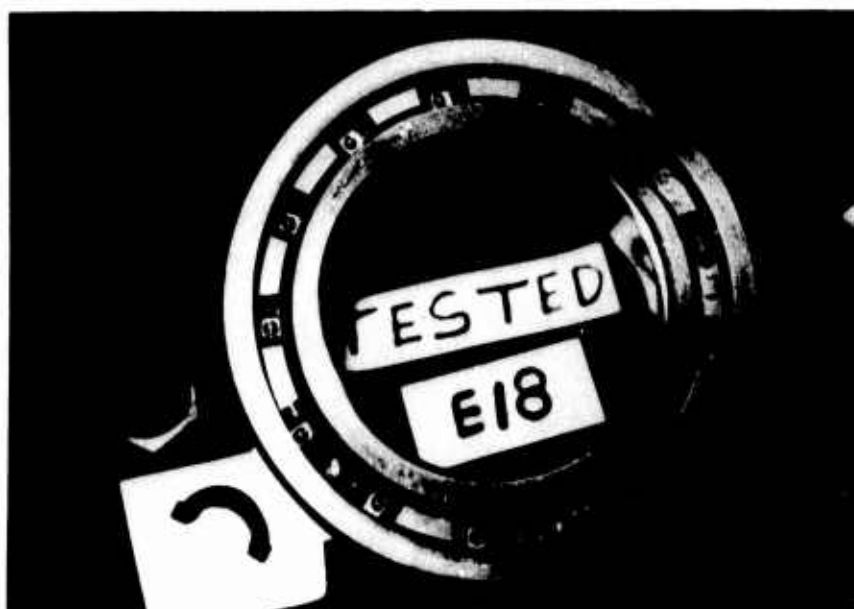
Figure 62. Bearing E18 After Failure, Test 10.
