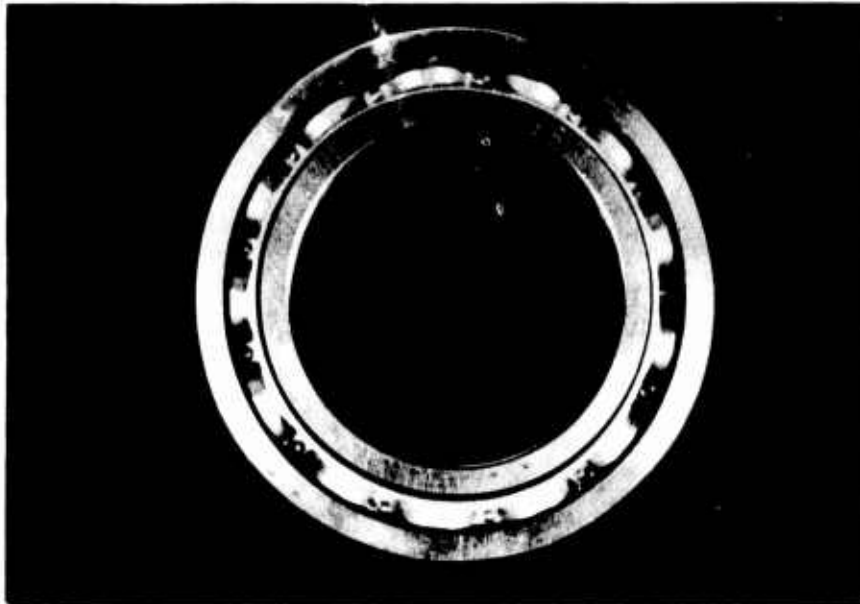
Figure 52. Bearing E14 Before Test (Cage Design 2).
