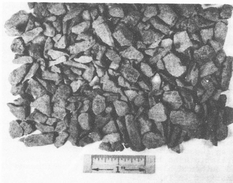
Figure 37. Typical Sample of Crushed Stone Injected Into Whirling Rotor.
