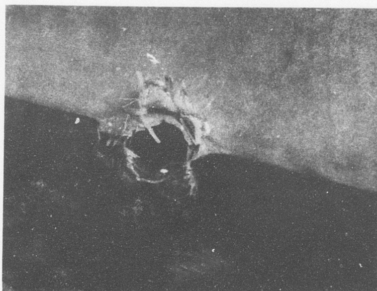
Figure 56. Ballistic Damage to B-Blade at Station 37.5 From 7.62mm AP Hit Through Forward Channel Section. (Bullet entered top surface as shown in upper view, penetrated through spar, and exited from bottom side as shown in lower view.)
