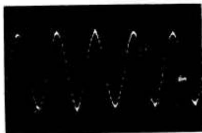
Test Accelerometer Output at 20-g Acceleration, 100-Hertz Frequency (Oscilloscope sensitivity is 0.5 V/cm vertically and 5 ms/cm horizontally.)
