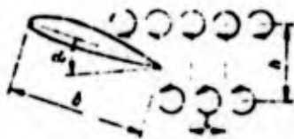
Figure 6.3. Diagram of the formation of a vortex street.
