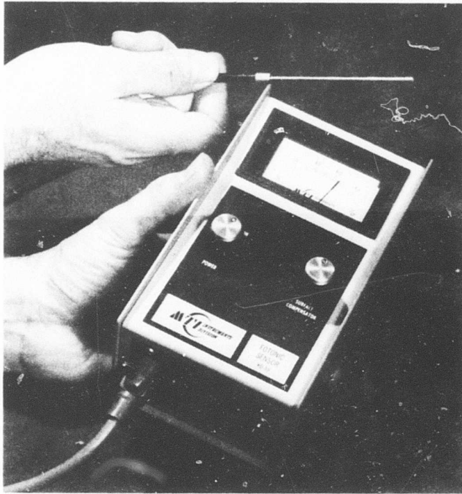
Figure 31. Fotonic Sensor-Optical Proximity Detector.
