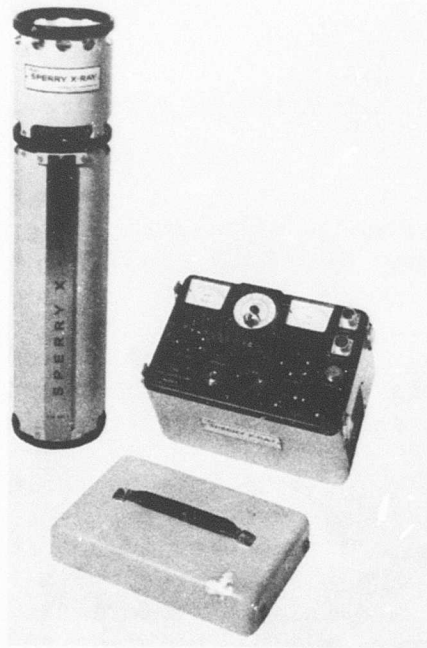
Figure 24. SPX 160 KV Portable Air Cooled X-Ray Unit.
