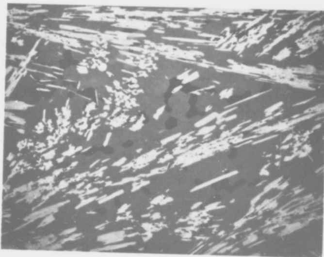
Figure 25. Hf-W-B (57/14/29): Alloy Arc-Melted and Subsequently Heat Treated at 1600°C for 300 Hours.
