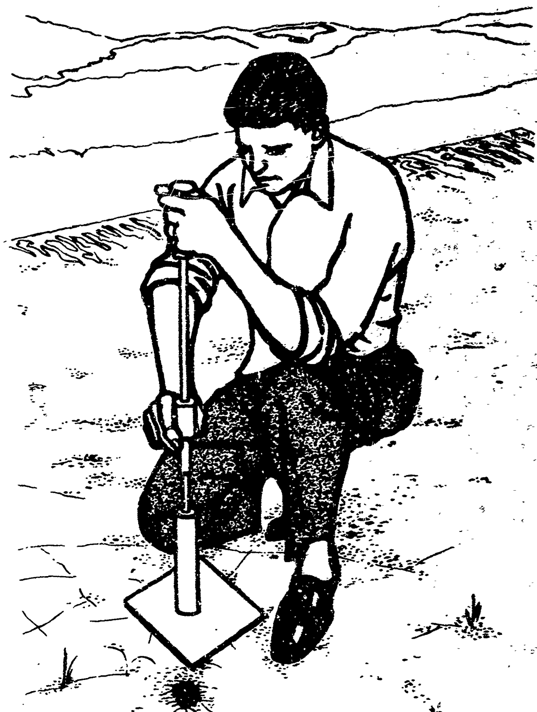
Fig. 9-5d. Applying Blows with Drop Hammer.
