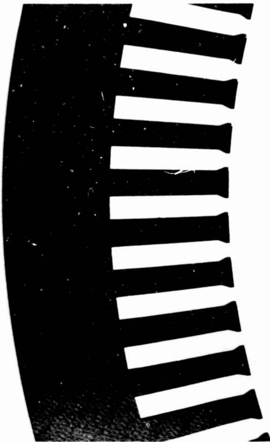
Figure 17. 0.004 Inch Stator Lamination Coated With Aluminum-Orthophosphate
