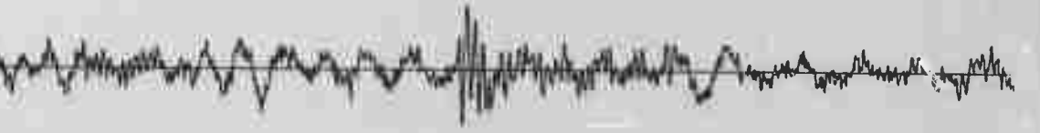
Figure IV-C. Deghosted Vertical Array Measurements, Method II (Reflection Coefficient 0.7)
