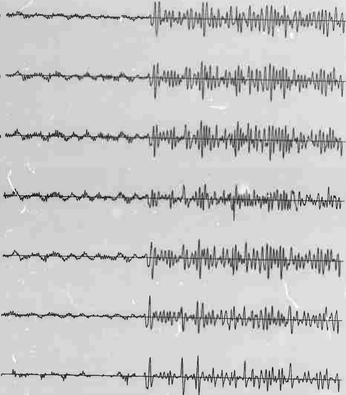
Figure I-A. Vertical Component Vertical Array Measurements--Aleutians, USCGS Focus 67 km, Magnitude 5.2, Date 6/17/65, Time 19:05:9.1
