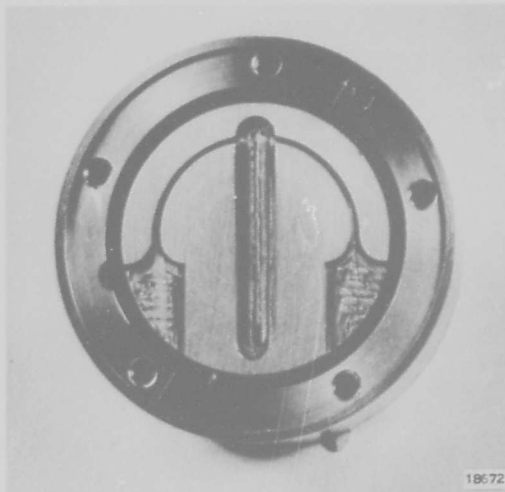
Figure 63 - View of the Transducer Showing the Rotor Ducts
